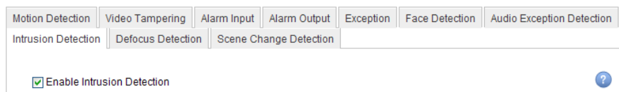
Figure 6. 12 Setting Intrusion Detection on IP Camera
